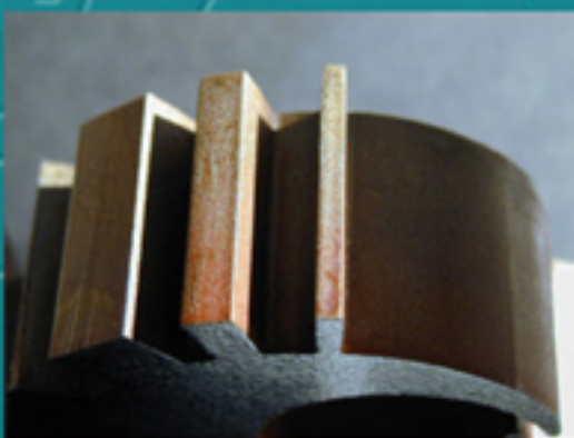
Part cut with Dynamic Waterjet™, showing elimination of taper
